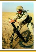
M224 Mortar Smooth bore, muzzle-loading, high-angle-of-fire weapon Unit Replacement Cost: \$10,658
